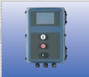
CS 300 pulse comfort control unit Microprocessor control unit with absolute encoder-evaluation. Simple but secure programming via 3-button navigation at the LCD monitor with multi-language plain text display, optional red-green "traffic light" indicator for door status messages, with optical warnings (application: e.g. underground car parks, car repair garages).
