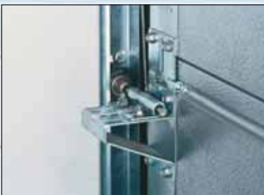
Low-noise operation Robust roller brackets made of galvanized steel and ball-bearing runners ensure that our doors run quietly and are durable.
