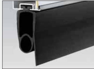
Bottom seal Non-perishable bottom seal made of elastic, anti-frost EPDM rubber profile compensates for any unevenness in the floor and offers protection from the cold and dampness.
