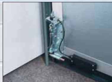
Bottom bracket For the bearer cable featuring integrated slack rope switch. Slight adjustment of door level at the bottom bracket (without spring shaft adjustment).
