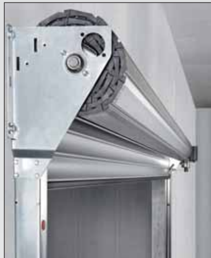
The roller shutter curtain is pre-assembled on the winding shaft and can be simply fitted into the console. The space saving console is bolted to the runner rail - no time-consuming measuring and marking required.
